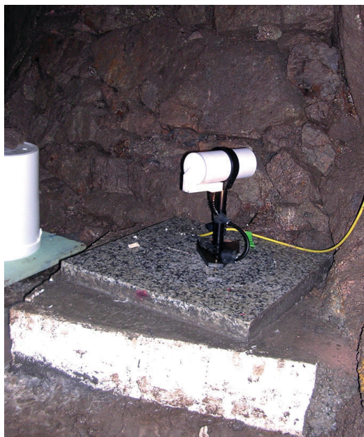
Figure 3.1: The Overhauser GSM-90 sensing unit installed in the upper tunnel of the Anton mine. The white cover (seen on the left) has been removed for the picture.
