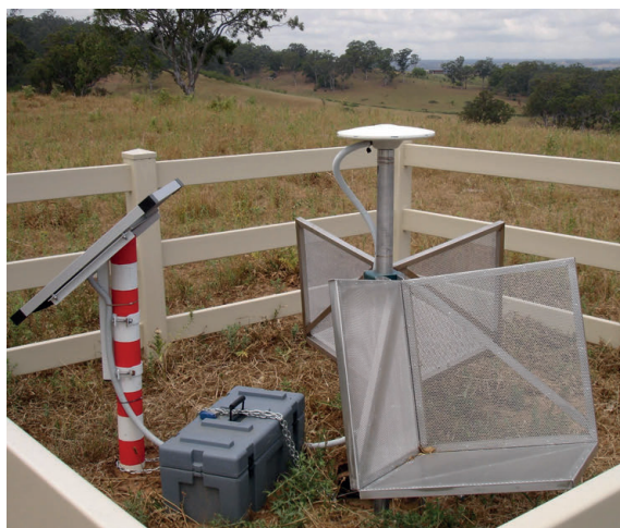
Figure 2.1: Geodetic monitoring site CA19 consisting of GNSS antenna/receiver and two CRs aligned for ascending and descending passes of Radarsat-2
