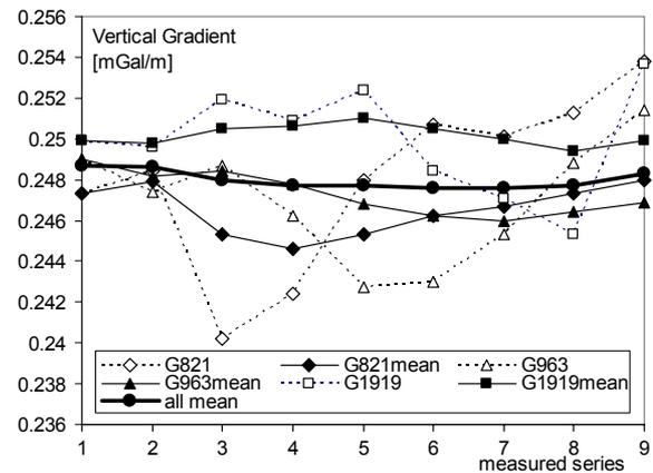
**Fig. 2** VG values by linear approximation from measurements at three different heights
