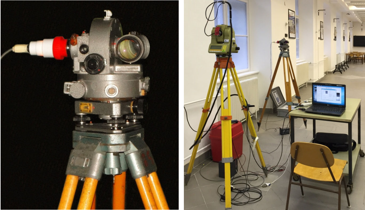
Fig. 5 The ATK-2 collimator and the laboratory test of the calibration with ATK-2 collimator
