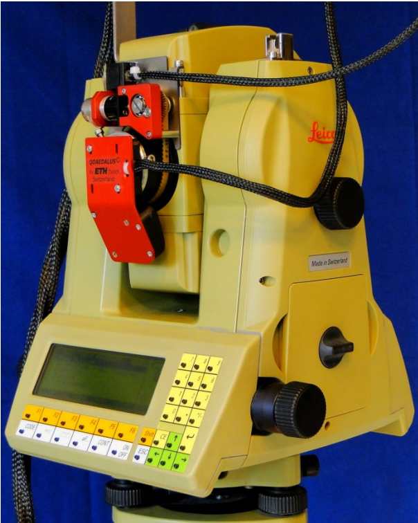
Fig. 1 Modified Leica TCA1800 total station with CCD sensor
