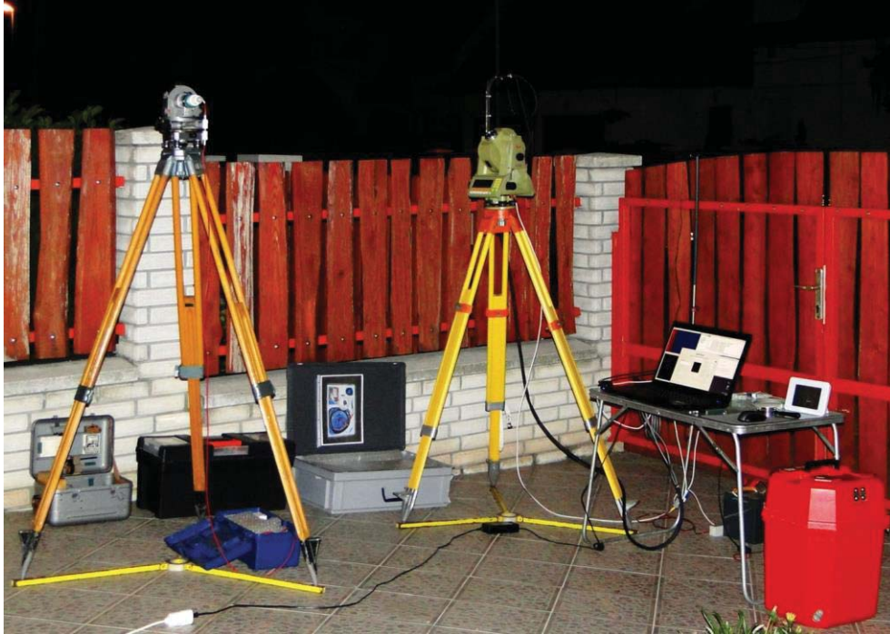
Figure 2. Night measurement by the Qdaedalus system at the point Pistahegy
