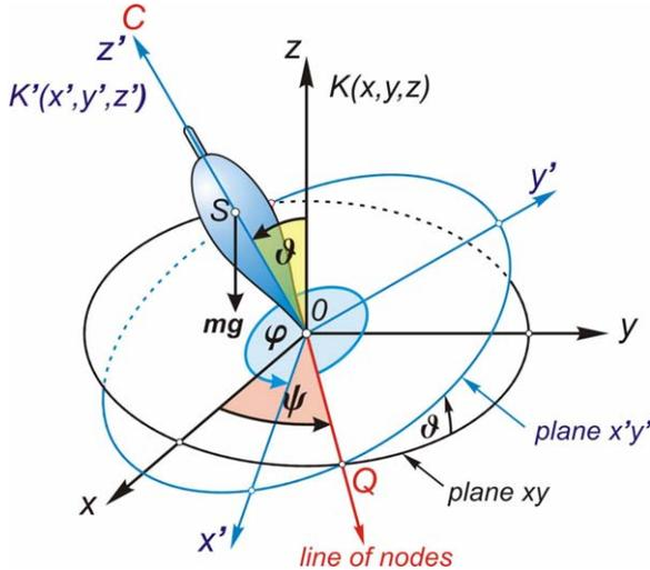
Fig. 2. Coordinates used to describe the motion of the heavy gyroscope
